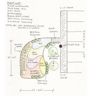
Water Resources Program, a rain garden, or bioretention system, is a landscaped, shallow depression that captures, filters, and infiltrates stormwater runoff at the source (Green Infrastructure Guidance Manual, 2016).
